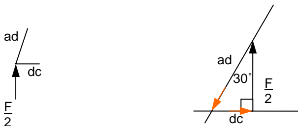
Close up of Joint ADC
